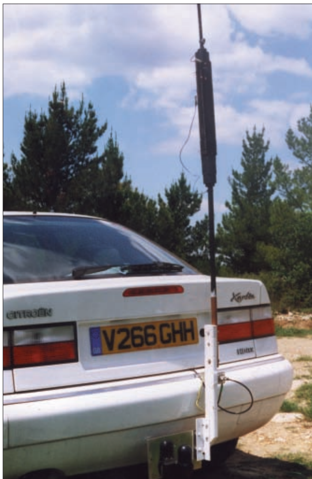
● Fig. 5: Full end-on view of MOEJB's car with the Midge Catcher in place and operational. Note the flying leads for selecting tapping points. See text for mounting and attachment suggestions.
